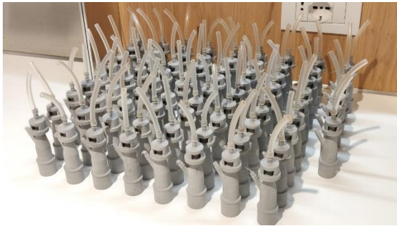
Figure 4 Respiratory valves designed and printed in just 24-hours [29]
