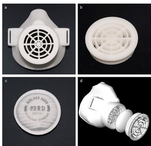
Figure 15 (a) Custom-made individualized 3D printed protective face mask, (b) filter membrane for support, (c) polypropylene (PP) non-woven melt-blown particle filter, (d) Three-Dimensional image of the prototype [54]
