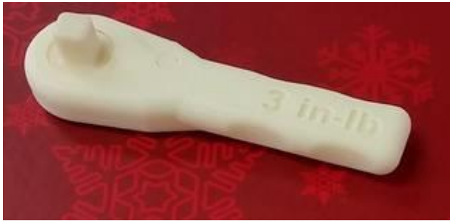
Figure 3 Wrench printed in space on the International Space Station [28]
